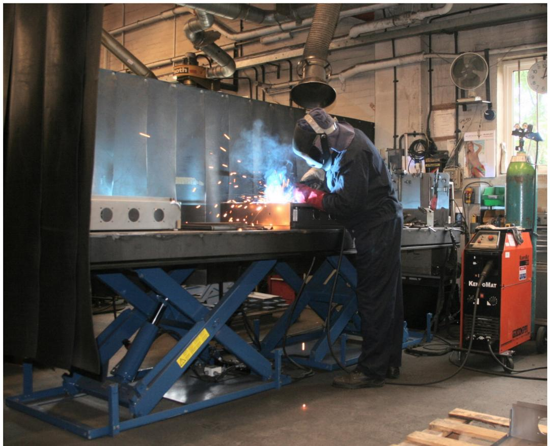
Picture shows welding bench with long platform to fit customer specific requirements. This table is based on a tandem scissor table because of the length. Platform 3000 x 1050 mm and 500 kg capacity
